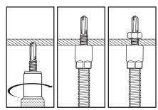
Install with appropriate sized steel socket driver.
