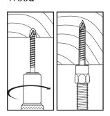
Install with appropriate sized wood socket driver.
